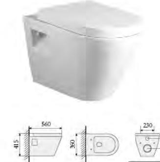
YS22236H-U Wall-hung closet, white UF seat cover, soft-closing P-trap, wash-down Size: 560x360x415mm
