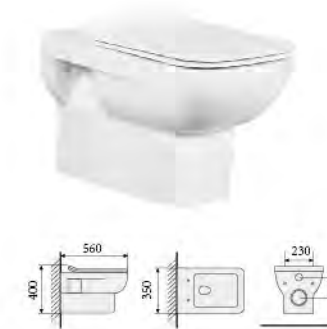
YS22233H-U Wall-hung closet, white UF seat cover, soft-closing P-trap, wash-down Size: 560x350x400mm
