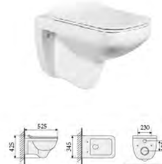
YS22212H-RU Wall-hung closet, white UF seat cover, soft-closing P-trap, wash-down Size: 525x345x425mm
