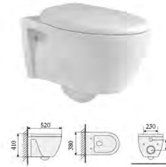
YS22244H-P Wall-hung closet, white PP seat cover, soft-closing P-trap, wash-down Size: 520X380X410mm
