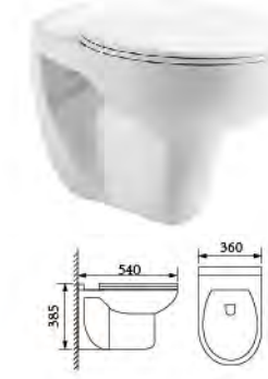
YS22269H-RP Wall-hung closet, white PP seat cover, soft-closing P-trap, wash-down Size: 540x360x385mm
