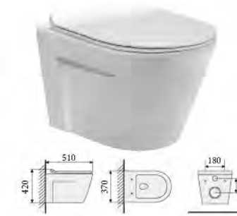
YS22267H-RU CE Wall-hung closet, white UF seat cover, soft-closing P-trap, wash-down, full open Size: 510x370x420mm
