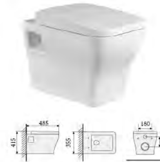
YS22245H-P Wall-hung closet, white PP seat cover, soft-closing P-trap, wash-down Size: 485X355X415mm
