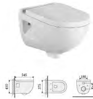
YS22203H-U Wall-hung closet, white UF seat cover, soft-closing P-trap, wash-down Size: 545x375x410mm
