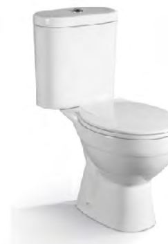
YS22206P/S 2-piece wash-down closet, white PP seat cover 3/6L dual flush valves Size: 660x360x760mm P-trap, 180mm roughing-in S-trap, 200mm roughing-in
