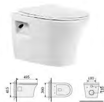
YS22278H-RU2 Wall-hung closet, white UF seat cover, soft-closing P-trap, wash-down Size: 495x360x415mm
