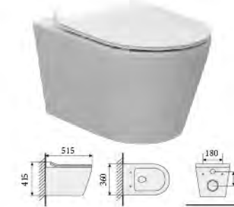
YS22268H-U CE Wall-hung closet, white UF seat cover, soft-closing P-trap, wash-down Size: 515x360x415mm
