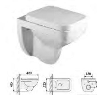
YS22287H-P Wall-hung closet, white PP seat cover, soft-closing P-trap, wash-down Size: 480x320x415mm
