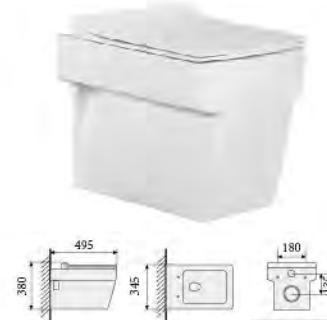
YS22243H-U Wall-hung closet, white UF seat cover, soft-closing P-trap, wash-down Size: 495X345X380mm
