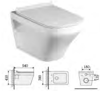
YS22249H-U Wall-hung closet, white UF seat cover, soft-closing P-trap, wash-down Size: 540X380X410mm
