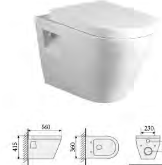
YS22236H-P Wall-hung closet, white PP seat cover, soft-closing P-trap, wash-down Size: 560x360x415mm
