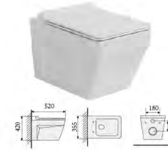
YS22281H-RU Wall-hung closet, white UF seat cover, soft-closing P-trap, wash-down Size: 520x355x420mm
