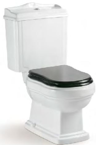
YS22209P/S 2-piece wash-down closet, white PP seat cover 3/6L dual flush valves Size: 670x445x860mm P-trap, 180mm roughing-in S-trap, 250mm roughing-in
