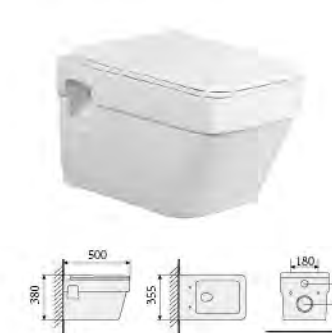
YS22285H-U2 Wall-hung closet, white UF seat cover, soft-closing P-trap, wash-down Size: 500x355x380mm
