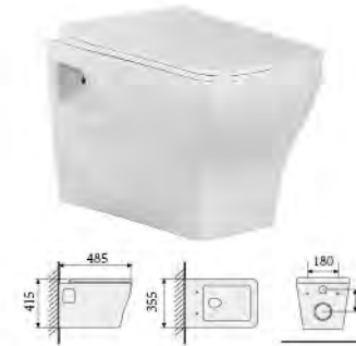
YS22245H-U2 Wall-hung closet, white UF seat cover, soft-closing P-trap, wash-down Size: 485X355X415mm
