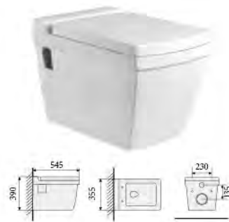
YS22242H-P Wall-hung closet, white PP seat cover, soft-closing P-trap, wash-down Size: 545X355X390mm
