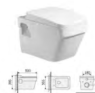
YS22285H-P Wall-hung closet, white PP seat cover, soft-closing P-trap, wash-down Size: 500x355x395mm
