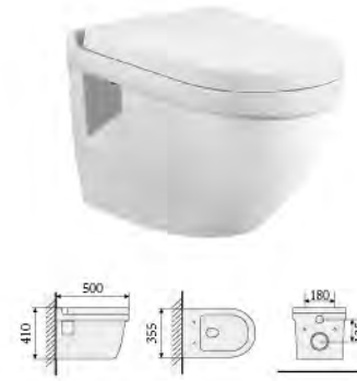
YS22210H-U Wall-hung closet, white UF seat cover, soft-closing P-trap, wash-down Size: 520x355x410mm
