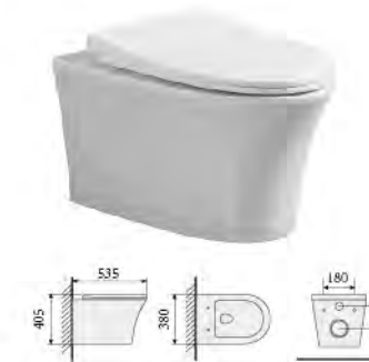
YS22283H-RP Wall-hung closet, white PP seat cover, soft-closing P-trap, wash-down Size: 535x380x405mm
