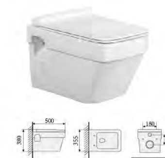
YS22285H-U Wall-hung closet, white UF seat cover, soft-closing P-trap, wash-down Size: 500x355x380mm
